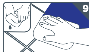
Lightly clean off excess adhesive with damp sponge
