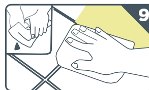
Lightly clean off excess adhesive with damp sponge
