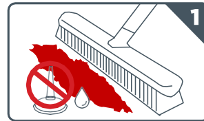
Clean surface of contaminants
